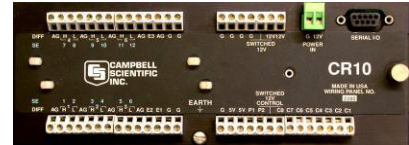
A multi channel programmable data logger (Campbells CR10).
