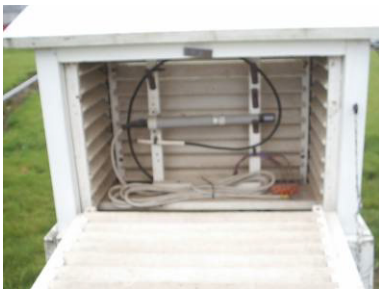
The wooden Stevensons screen is the world standard screen for meteorological observations.
