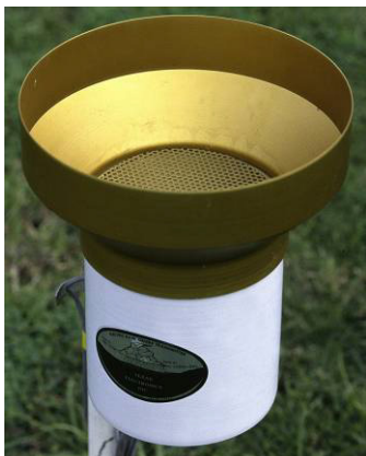
Tipping bucket rain gauge with wide collection funnel used for 0.1mm tipping increments.
